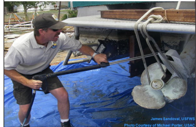
Figure 10. Decontamination of a Houseboat
