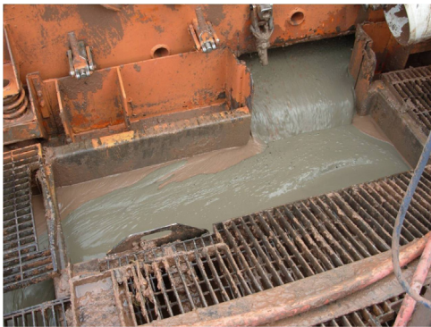
Figure 16. Gray Cement Starting to Emerge from the Annulus
